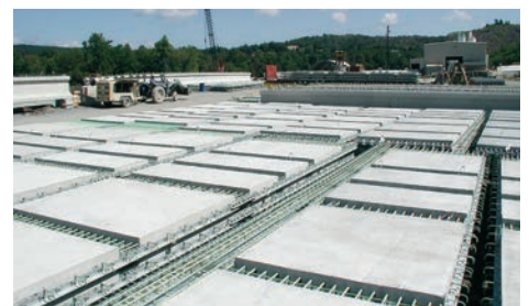
Precast grid deck panels.
