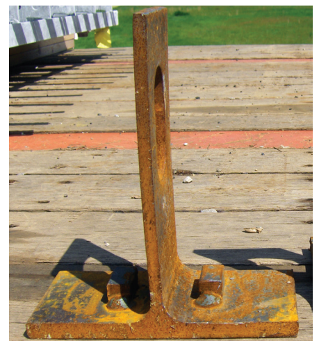
Lifting device made from WT shape.
