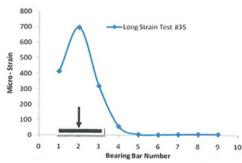
Figure 1: Results are from test on 37R5 Lite 5" x 1/4" riveted steel deck. Maximum response is from the three bearing bars directly under the sumulated tire patch. Main bars are spaced at 5.125" on center.
