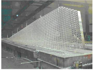
Hot-Dip Galvanized Grid Deck Panel
